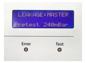
In contrast to the instructions supplied by the manufacturers of the endoscopes, the pretest is performed with the endoscope not moving and preferably fully extended. In this way, the pretest will also detect microperforation.
